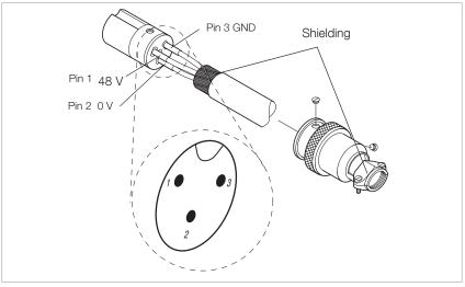
Fig. 3.16 Reqired pin assignment of the 3 pole connector model Hirose HS21P-3; view from the soldered side
