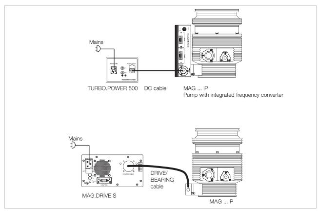
Fig. 1.11 System configurations
