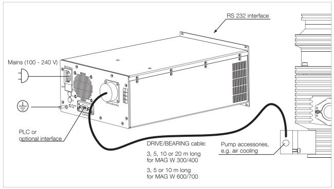
Fig. 3.18 Connection schematic MAG.DRIVE S
