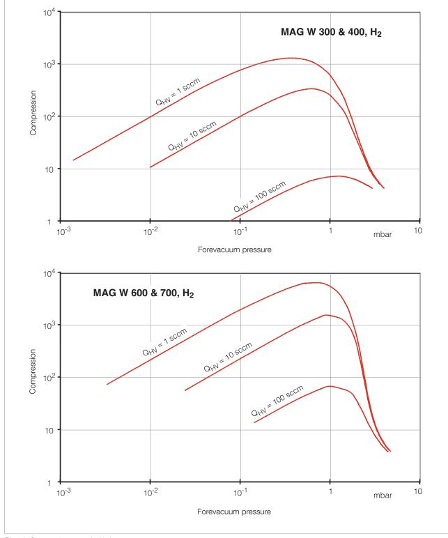
Fig. 1.6 Compression curves for Hydrogen
