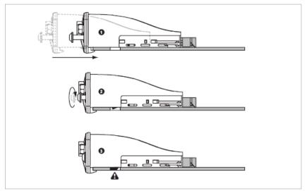
Fig. 4.2 Installation of an interface module
