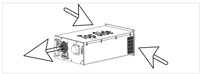
Fig. 3.19 Air flow pattern for MAG.DRIVE S
