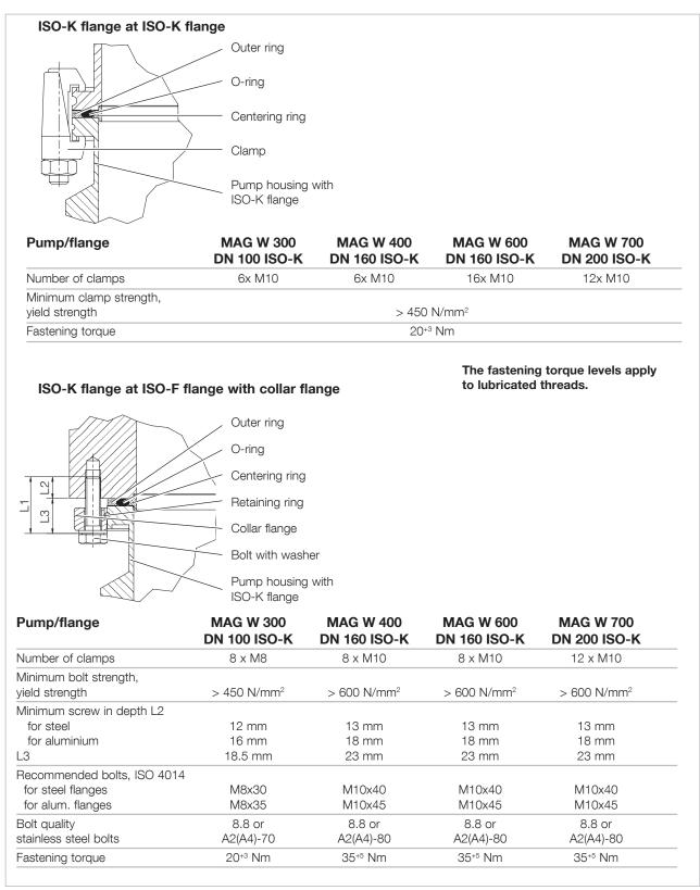
Fig. 3.4 Mounting high vacuum flange ISO-K.
