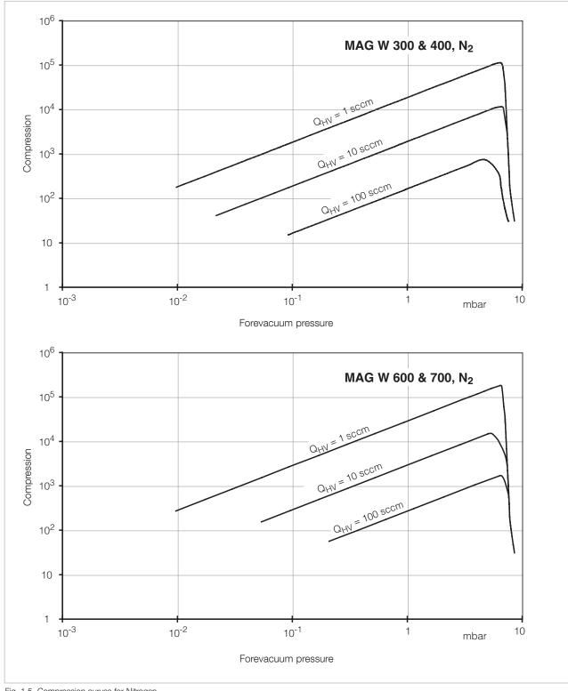
Fig. 1.5 Compression curves for Nitrogen
