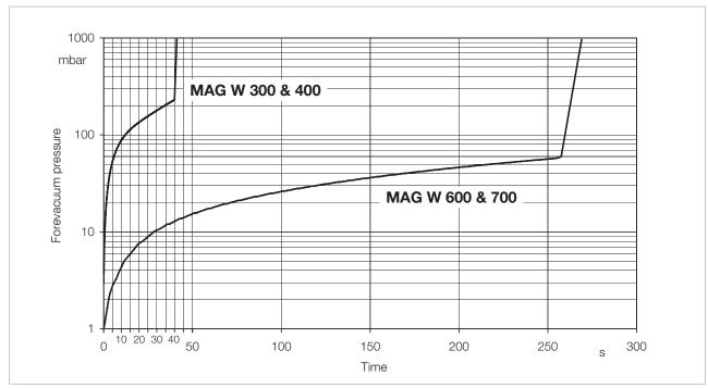
Fig. 4.4 Pressure rise curve for safe venting
