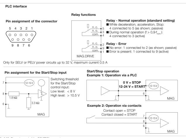
Fig.3.20 Pin assignment of the CONTROL connector
