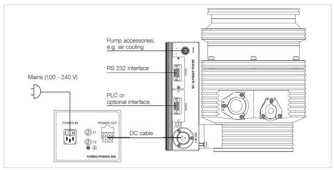
Fig. 3.14 Connection schematic TURBO.POWER 500 power supply
