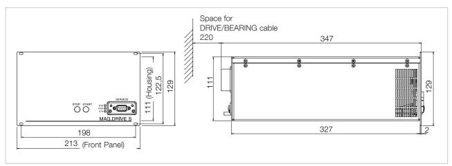
Fig. 1.10 Dimensional drawing of the MAG.DRIVE S, dimensions in mm
