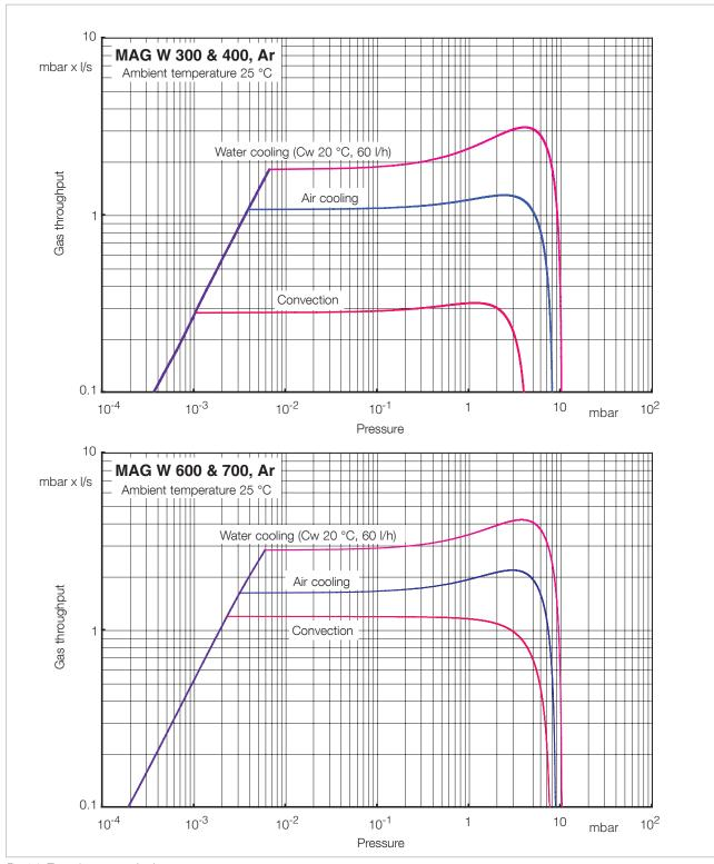
Fig. 1.8 Throughput curves for Argon
