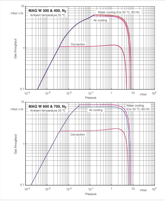
Fig. 1.7 Throughput curves for Nitrogen
