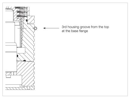
Fig. 3.11 Mounting position of the water cooling
