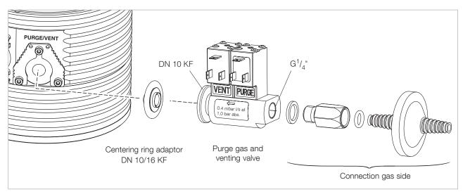
Fig. 3.13 Connect purge gas and venting valve
