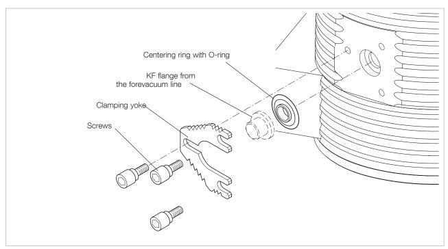
Fig. 3.7 Connecting the forevacuum line
