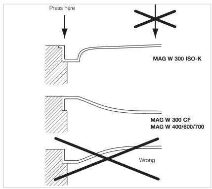
Fig. 3.3 Installing the inlet screen
