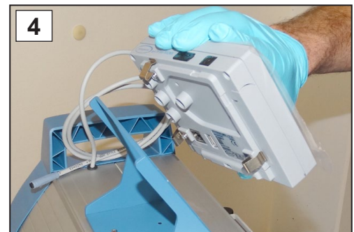
4. Clip the controller into the base.
