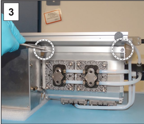
2. Wind the screw fittings into the side panel; hex key size 5.
