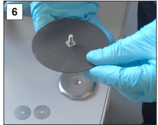
6. Place the new diaphragm over the square head of the clamping disc.
