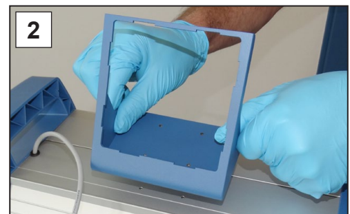
2. Position the base on the diaphragm pump.
