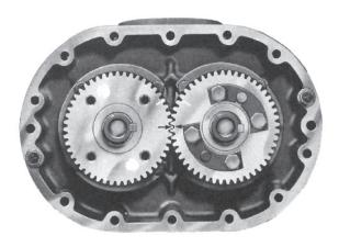
Figure 10-2 – Keyways in line and timing marks matched
