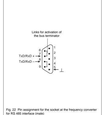
ISO 8482, EIA 485 Protocol acc. to VDI/VDE 3689 Transmission rate 19200 baud fixed Response delay default setting 10 ms (parameter 180)
