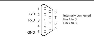
Fig.20 Pin assignment for the socket at the frequency converter (female)
