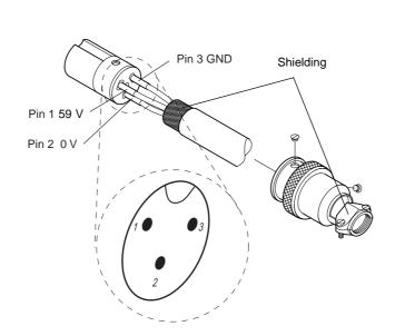
Fig. 17 Reqired pin assignment of the 3 pole connector model Hirose HS21P-3; view from the soldered side
