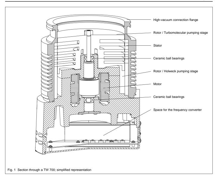
The pump is driven by a canned DC motor. In this motor the rotor and stator windings are separated by a vacuum-tight can. Consequently the rotor runs inside the vacuum while the stator is outside the vacuum. This eliminates any need of vacuum feedthroughs.
