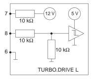
Switching threshold for the Start/Stop control input: Low level: < 3 V High level: > 7 V
