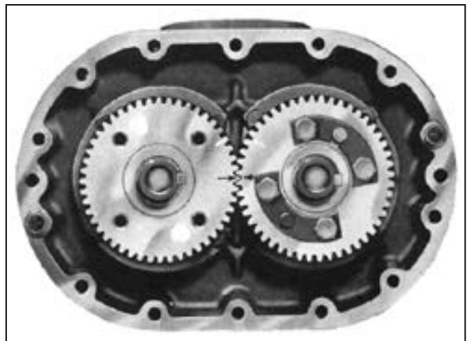
Figure 9A - Keyways in line and timing marks matched
