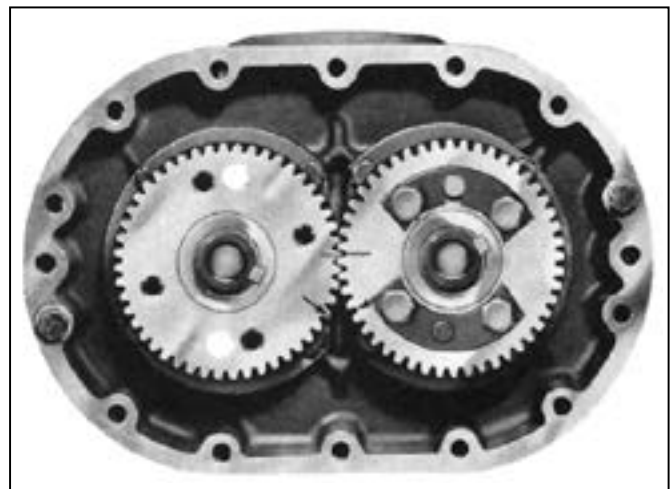
Figure 9B - Timing marks advanced 3 teeth (Reference marks aligned)
