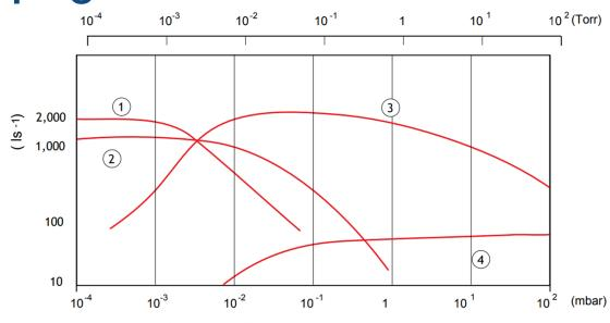
In their most efficient range mechanical booster pumps (3) cover the gap between oil vapour diffusion pumps (1), Oil vapour booster pumps (2) and rotary or dry primary pump (4)
