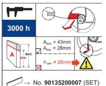
After 3000 hours of run time on the pump, the vanes will need to be checked for wear. To open vane location area, remove metal end cover, unscrew bolts.
