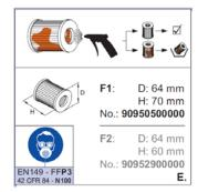
There are internal filter/elements. Every model has a filter behind the front face plastic shroud or an external filter on the inlet side of the pump (F1). In some pump types, there will also be an internal exhaust filter. (F2)
