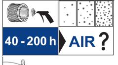
Filter/elements should be checked between 40-200 hours. The elements should be blown with compressed air from the inside out. Blast air should be felt coming through the filter/element. The element needs to be replaced if dirty or clogged. Use only Becker Genuine filters to maintain warranty protection.
