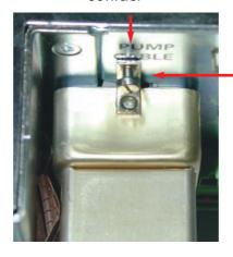
Caution: If the two surfaces aren't in contact, it means that the connector is not in well installed, an electrical damage can occur.
