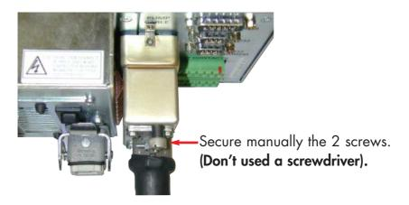
Assemble the two small screws that you had previously disassembled and check that the surfaces are in contact with the ACT.
