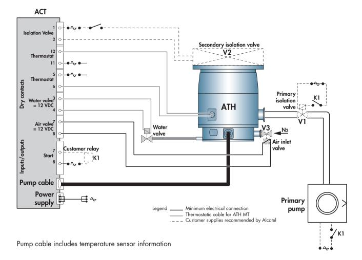
Wiring diagram in case of temperature regulation with the controller
