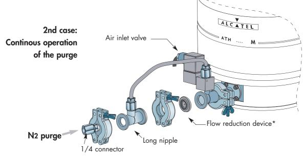
\* 50 SCCM: standard furniture. 25 SCCM: upon request (accessory) Connect the little flexible pipe between the long nipple and the valve.
