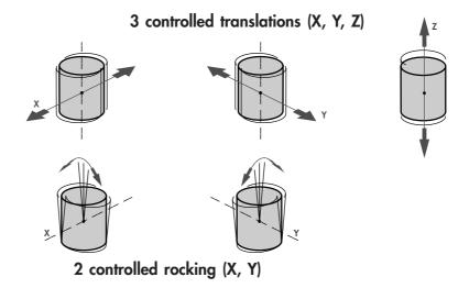
Movements in relation to these axes are monitored by position sensors. According to the position data recorded, the ACT controller corrects differences to bring the rotor back to its optimum position, by varying the current in electro-magnets.
