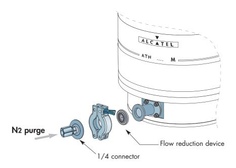
Connect the nitrogen supply to the DN 16 purge fitting\*. The nitrogen flow reduction device controls the pressure and guarantees a flow rate of 50 SCCM at pressure 1.1 bars.
