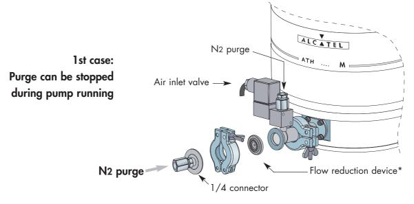
Note: N2 supply can be equipped with massflowmeter and, in this case, it is not necessary to install the flow reduction device.
