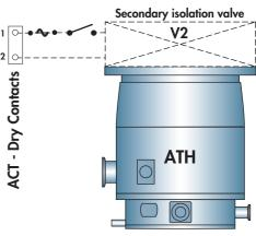
contact opens and closes the secondary isolation valve.
