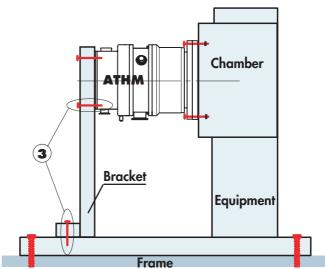
The equipment frame on which the pump is installed must be sufficiently rigid to absorb the kinetic energy of the rotor in case of pump rotor crash. For this, take into account:
