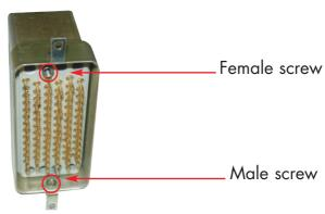
Plug the connector accordingly and press the connector axially, tighten **manually** the 2 screws at the same time (**Don't use a screwdriver**).
