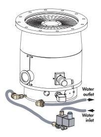
CAUTION Avoid to screw the connector on the valve inlet port using a 13 mm flat wrench, to maintain it (water leak risk).
