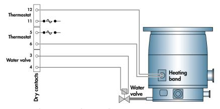
Connect the water valve via the «WATER VALVE» contact on the DRY CONTACTS connector.
