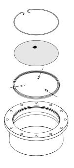
Orientate the filter-holder (2) according to the way of mounting described as follows (chamfer looking to the inside of the pump) and position it into the inlet housing.
