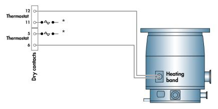
Connect the heater cable via the «THERMOSTAT» contact on the DRY CONTACTS connector and to the power line (110 or 230 VAC).
