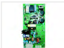
* D001 P0330E1 POWER SUPPLY BOARD - 142/182
