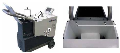
It the leak detector is equipped with the bottle holder accessory, accessories in the inlet port or other customization, remove it (them) before beginning detector packaging.
