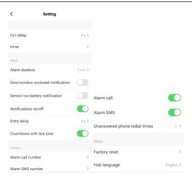
• Exit delay – Your security system has been programmed with delay times that allow you to exit your home after arming. If you leave home too late when exiting, it will cause a false alarm. If a false alarm occurs, you should disarm the system immediately. Tap on Exit delay to change the amount of delay time you have to leave your home; choose how many seconds you wish to delay the alarm setting and remember to confirm so that the new setting is saved.
