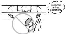
Never wash the air conditioner with water. Otherwise electrical shock can occur.
