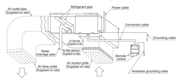
Model FXDQ~SPV1 (Example: When the air is supplied from the back)
