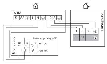
ERWQ02AAV3 Exterior heat pump unit X1M Terminal rail on EKHHP
