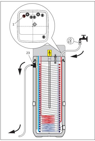
Fig. 9-1 Filling the storage tank - without solar system
