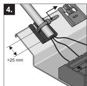
Fig. 4-9 Click the holding clip in place and retain the cables with the ca-
