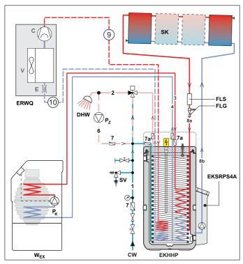
Fig. 4-5 Hydraulic connection - legend see tab. 4-2 (Example EKHHP500A\*2V3 with PO Solar and optional external heat generator)
