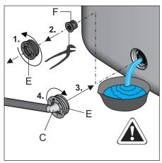
Screwing pre-assembles connector into the filling and draining connection
