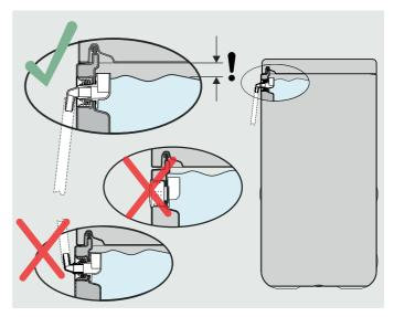
Installation of drain hose at safety overflow
