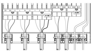
Fig. 4-8 Tension relief using cable ties
