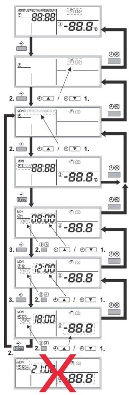
Fig. 7-3 Delete individual switching times
