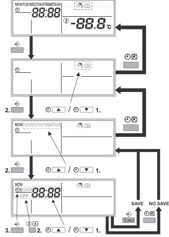
Fig. 7-2 Display and programme switching times
