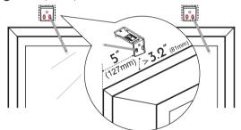
6 Drill holes & install mounting brackets.
