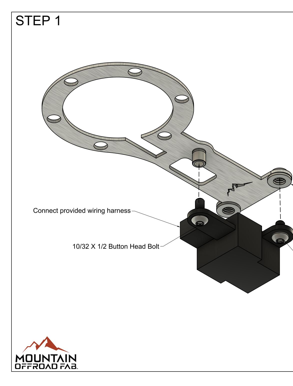
Start by first connecting the provided harness to the switch module. Next you will attach your factory Jeep cruise control switch to the bracket using the provided 10-32 Stainless Steel hardware.
