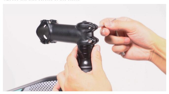
2.Strip off the cover, use the Allen wrench to loosen the top screw.
