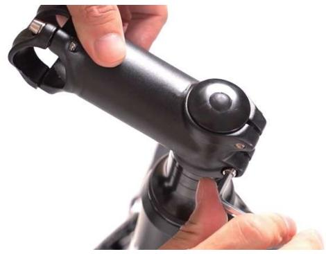
4 Loose the all the 4 screws of the stem and install the the handlebaron it. Then adjust its position before fix it with the screws
