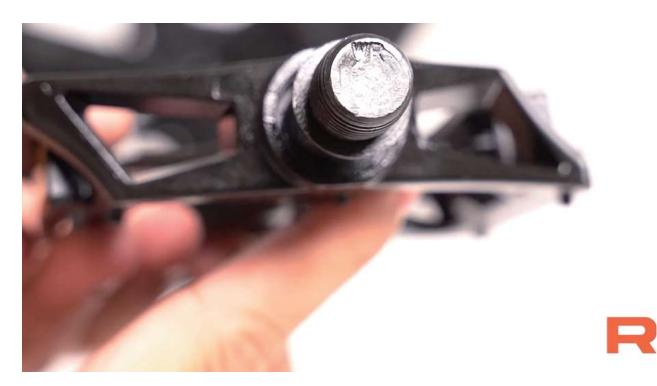
2. Install the right pedal on the right crankset and rotate it CLOCKWISE to tighten.(Counterclockwise for the left pedal)
