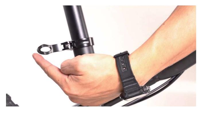
3.Adjust the seat to a suitable height and lock the seat post clamp.
