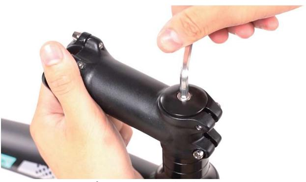
3.Rotate the stem 180° to the opposite direction, and then tighten the side and top screws.
