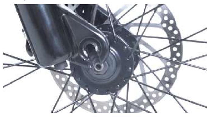
2. Use the quick release lever to assemble the front wheel. Remember to put on the spring when installing.
