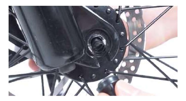
3. Loosen the quick release on the other side before buckling it, so that it is unable to be fastened because the other side is too tight.
