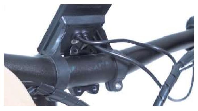
2. Holding the faceplate on the stem and tightening the four screws with hex wrench provided.
