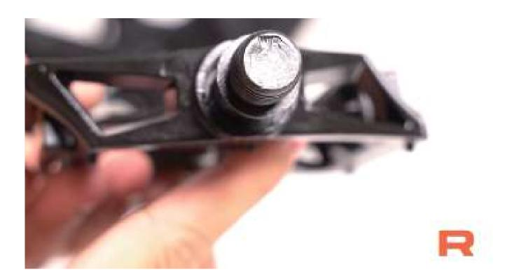
2. Tighten spindle end, don't turn the pedal to tighten.
