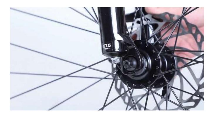
4. Continue to adjust the quick release and nut until they are locked.
