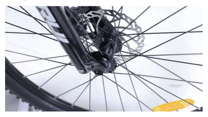
2 . Insert the quick release into the hub , note that only one spring on each side.
