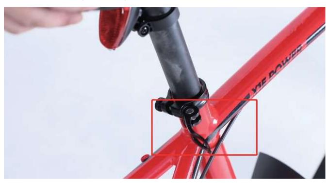
2. Insert the seat post into the frame tube.
