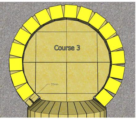
Using the chamber template as a guide from the centre of the oven rotate it around and lay your bricks in the pattern for the second layer Make sure you lean the bricks against the template guide to correctly set the angle
