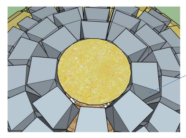
For the keystone mix some CAST 13 in a bucket and pour into the top to lock the entire structure togther.
