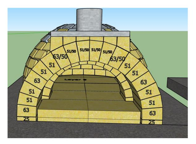
Screw the flue arch template together using 180mm timber battens and build your flue arch.
