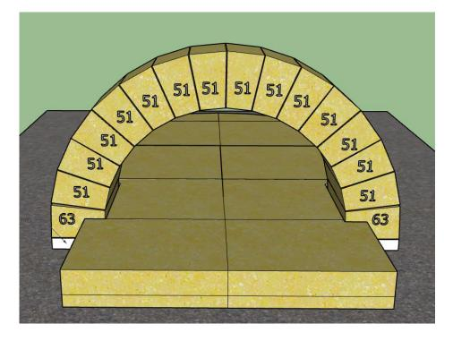
When you have finished the door arch leave the template in for at least an hour before removing it. You can also leave it in while building the chamber if you like.
