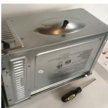
Smear the beads to glue to better seal the gaps, and help the glue cure faster. The front corners of the oven, and the gaps around the heating elements are closed too.
