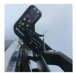
The door servo is always moved to the closed position when the oven powers up. Typically, the door will be opened slowly soon after the maximum temperature is reached, and closed again when the oven cools to 50°C. You can change that behavior in the reflow profile though.
