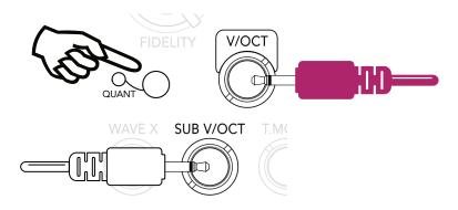
V/Octave pitch control is available for the main wavetable and the sub oscillators. Connections are standard mono  $3.5 \text{mm} / 1/8^{\text{th}}$  TS jack patch cables
