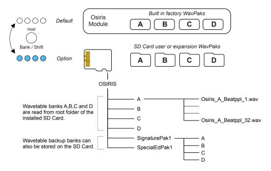
The WavPak to be used should be located in the SD card root within the 'OSIRIS' folder. If required. additional WavPaks may be held on the SD card located in backup folders for storage. Any backup wavetable that are then required to be used can be copied from the backup to the SD Card root folder with a PC or Mac.
