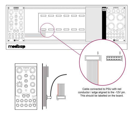
Cable connected to module with correct orientation with red conductor / edge aligned to the -12V pin. This should be labelled on the module board with a white dash...
