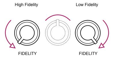
Fidelity setting can be manually adjusted across the range between the high to low settings using the rotary control or modulated with a connected CV into the fidelity input
