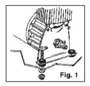
PLEASE NOTE: DO NOT OVER TIGHTEN THE BRAIDED COMPRESSOR AIR HOSE FITTING, AND OTHER FITTINGS IN SYSTEM! BY OVER TIGHTENING FITTINGS, IT MAY CAUSE A SMALL AIR LEAK IN THE SYSTEM. WHEN THE AIR COMPRESSOR LOSES AIR CONSTATLY, IT WILL COME ON MORE OFTEN TO REPLENISH THE LOST AIR, AND EVENTUALLY GET HOT AND BREAK DOWN, AND SHORTEN THE LIFE SPAN ON THE COMPRESSOR. FITTING SHOULD BE TIGHTENED SNUG!
