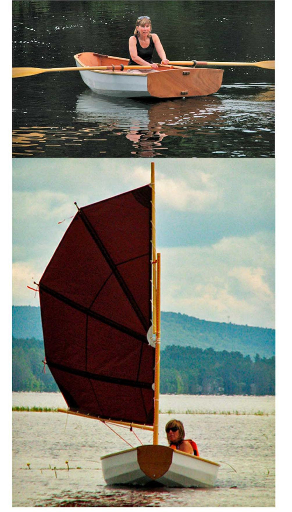
detonthewater.ca This boat is based on the Norweigian style of pram. intended to be used both for rowing and sailing. Built using the stitch and glue method. As we do with all our small sailing designs we design the sail plan based on readily available kits from Sailrite so the builder can complete their own sail.
