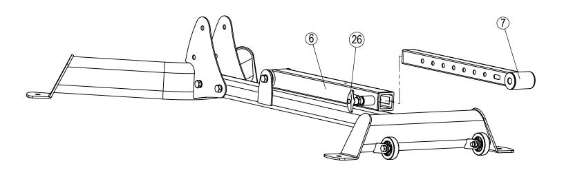
A Loosen the Pop-pin (26) and insert the Lower Adjustment Tube Assembly (7) into the Pivot Tube Assembly (6).
