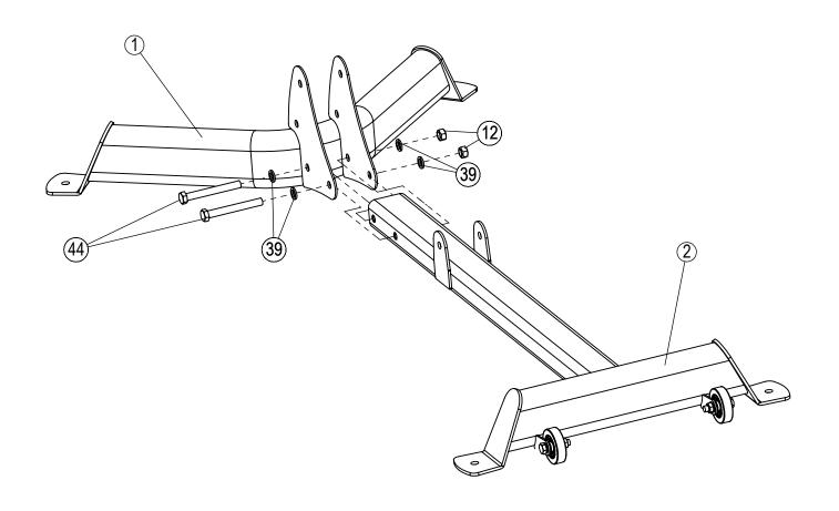
A Combine the Front Foot Tube Assembly (1) and the Stabilizer Assembly (2) using 2- Hex Bolts M12x100 (44), 4- Flat Washers \$\phi\$12 (39), and 2- Lock Nuts M12 (12).
