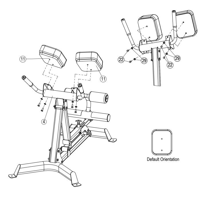
A Attach the Back Pad Assembly (11) onto the Handle Assembly (4) using 2- Hex Bolts M10x25 (22) and 2- Flat Washers  $\phi$ 10 (29). Repeat for both sides.
