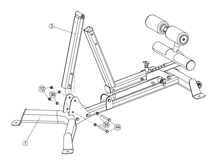
A Attach the Front Support Tube Assembly (3) to the Front Foot Tube Assembly (1) using 2- Hex Bolts M12x100 (44), 4- Flat Washers \$\phi\$12 (39), and 2- Lock Nuts M12 (12).
