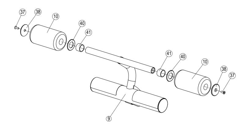
A Attach the Aluminum Cap (38), Foot Roller (10), Plastic Washer (40), and Foam Stopper (41) to the Leg Rest Assembly (9) using 1- Flathead Screw M10x25 (37). Repeat for both sides.
