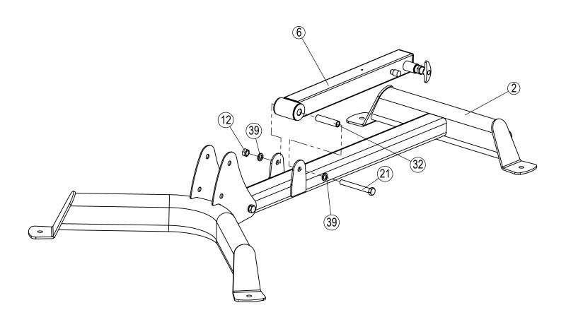
Attach the Pivot Tube Assembly (6) to the Stabilizer Assembly (2) using 1- Hex Bolt M12x95 (21), 2- Flat Washers  $\phi$ 12 (39), and 1- Lock Nut M12 (12). Make sure the Hex Bolt M12x95 (21) goes through Spacer 2 (32) inside the Pivot Tube Assembly (6).
