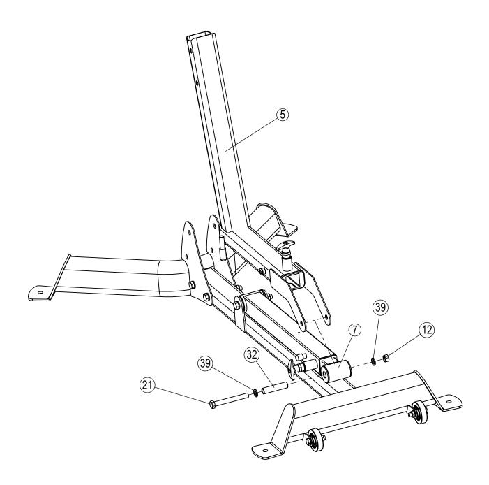
Attach the Adjustment Tube Assembly (5) to the Lower Adjustment Tube Assembly (7) usinge 1- Hex Bolt M12x95 (21), 2- Flat Washers  $\phi$ 12 (39), and 1- Lock Nut M12 (12). Make sure the Hex Bolt M12x95 (21) goes through Spacer 2 (32) inside the Lower Adjustment Tube Assembly (7).
