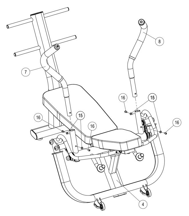
A Attach Left Handlebar Assembly (7) and Right Handlebar Assembly (8) to the Rear Support Assembly (4) using 2- M8x20 Hex Screws (15) and 2- M8 Flat Washers (16) on each side.
