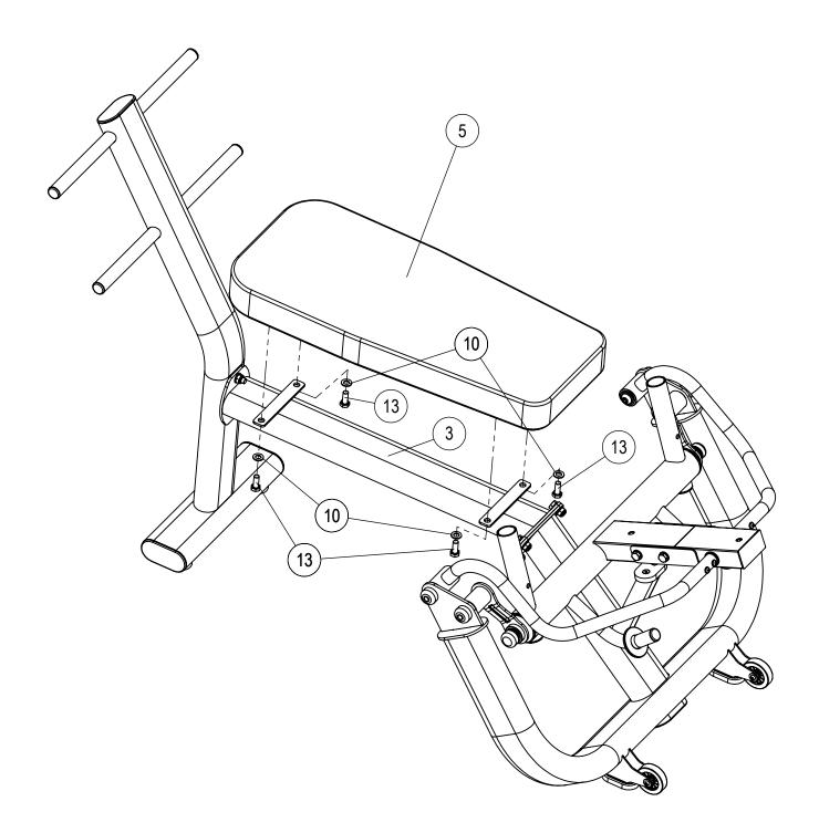
A Attach the Seat Pad Assembly (5) to the Seat Assembly (3) using 4- M10x25 Hex Bolts (13) and 4- M10 Flat Washers (10).
