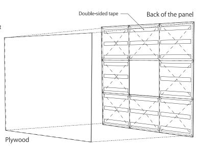
Drive screws from the back of the plywood into the panel mounting points.
