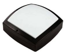
Housing: Die Cast Aluminum Housing and Open Front Frame, Textured Powdercoat Finish Over a Chromate Conversion Coating, Gasketed.
