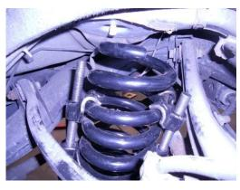
Using a set of spring compressors, compress the new spring approximately 1 inch then place the large end of the spring around the locator on the control arm.
