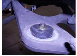
Make sure underside large washer is in the center of the control arm recess then tighten the nut and bolt.
