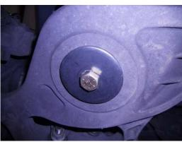
Prior to installing the spring, you will need to install the new shock into its upper mount inside the vehicle. Tighten the nuts.
