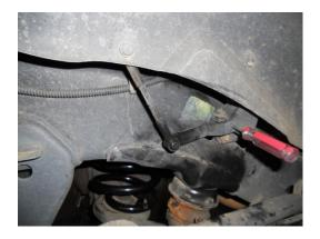
Remove the push pin install small wire tie to hold sensor arm in place. Re-install push pin.
