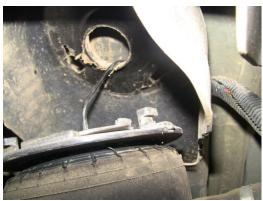
Remove the bottom rear shock bolt, using an 18 mm wrench and socket.
