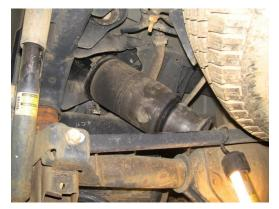
Cut the air line from the air spring. Remove the air spring from the vehicle.
