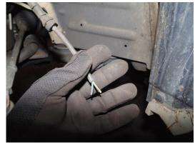
Strip the ends of both wires.
