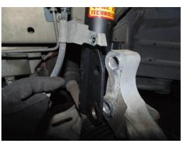
Align the struts lower mounting holes. \*Note\* It may be necessary to use a small pry-bar or large screwdriver to align the mounting holes.
