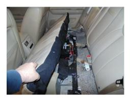
Disconnect the (-) negative cable from the battery using an 8mm wrench.
