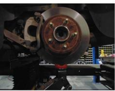
Using a 24mm socket and a 21mm wrench; loosen both of the struts lower mounting nuts. \*Note\* Only loosen the nuts to the ends of the mounting bolts.
