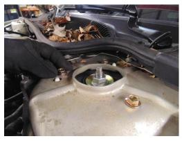
Place the bottom of the strut into position on the knuckle assembly.
