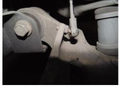
Support the lower a-arm and hub assembly with a floor-jack or lift support.
