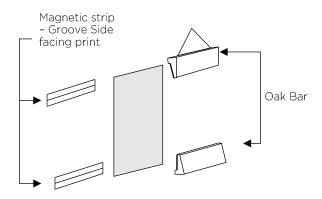
Sandwich your print or poster with the oak bar on the front and the magnetic strip (groove side down) placed on the back. The back of the oak has a magnetic strip already attached and if the removable magnetic strip is not used groove side down then it will not be strong enough to keep you poster or print in place.
