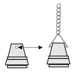
The two holes are for a chain to be attached and so the ceramic pull can be used as a cistern pull if required
