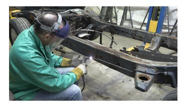
Clean the frame free of rust and debris revealing bare metal. Paint the work area with a weldable primer to help prevent against rust development.
