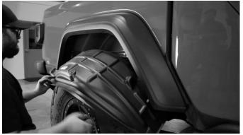
Inside the wheel well, at the shown hole, with an M8 Nutsert tool, install one of the included nutserts into the vehicle.
