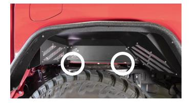
With a 3mm allen and two of the included M6 bolts, washers, and serrated nuts, secure the bottom of the fender.
