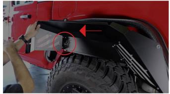
Slide your front inner fenders into the well and align the holes behind the body and into the nutsert.
