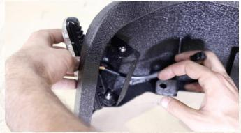
The alignment will be adjusted after the fender is installed.
