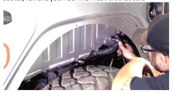
Gently pull the neck loose and push it down below the stud. The passenger side doesn't need to be changed.
