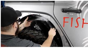
Tighten all visible bolts with a 3mm Allen key.
