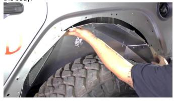
Tighten all visible bolts with a 3mm Allen key.
