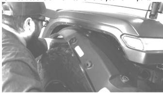
Within the driver side **rear** well, and with a 10mm socket, remove your fuel filler neck bracket bolt. Gently pull the neck loose and push it down below the stud. The passenger side doesn't need to be changed.
