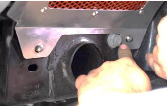
Tighten all visible bolts with a 3mm Allen key.
