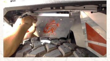
Secure the top with a 16mm bolt, washer, and nut.
