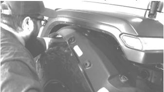
Within the driver and passenger **front** wells, and with a 9/32" drill bit, expand the two frame holes that are shown below.
