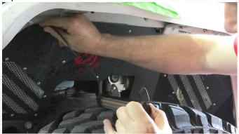
Insert the LED into the opening while being sure that the retaining flanges are on the outside of the fender brackets. Secure the brackets with the hardware that came with the Elite Fenders with a 3mm allen wrench and an 8mm wrench.
