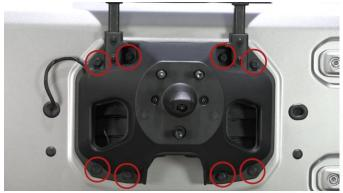
Using a 13mm Socket remove the eight tire carrier bolts. Using a T-25 Torx bit remove the backup camera retaining plate, pull the camera free from the backside of the tire carrier.
