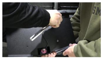
With the camera facing down place the Backside to the tailgate and secure it to the tailgate using the eight 13mm bolts.
