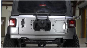
Using a T-40 Torx wrench remove your spare tires retaining clip. Next remove the three lug nuts and remove the vehicle's spare tire.
