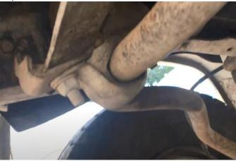
Drop the bar, brackets, and bushings, while retaining the factory hardware. Unless you decide to replace them, keep the bolts in the crossmember, as they will be reused in the next step.
