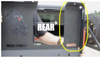
As shown above, this section will always face the rear of the vehicle, and the tub rail holes will cover your vehicle's rearmost rail holes.
