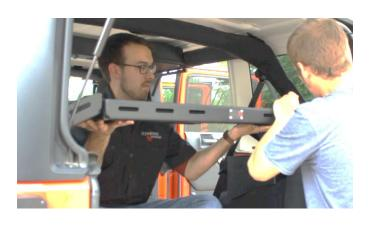
Secure each side with (3) Bolts, (6) M10 Flat Washers, and (3) Nyloc Nuts.
