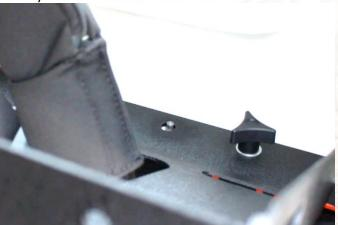
With your marker, mark the location of the forwardmost Support Plate hole that will be drilled out later.
