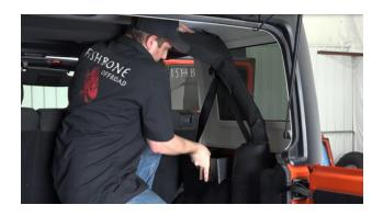
Either using all of your OEM hardware, or the supplied two (2) knobs and washers, secure the storage bin in place. Reuse your factory hardware to finish securing your hard top.
