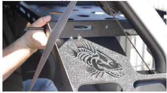
Secure each side with (3) Bolts, (6) Flat Washers, and (3) Nyloc Nuts.
