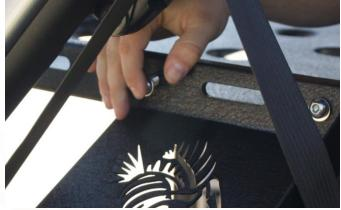
Tighten down the bolts with a 17MM Socket and a 6MM Allen wrench.
