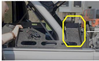
As shown above, this section will always face the rear of the vehicle, and the tub rail holes will cover your vehicle's (2) most rear rail holes.
