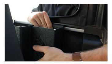
Push the bin's bracket under the pillar and over the bolt threads until it sits evenly with the tub rail.
