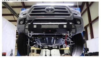
Begin removing your factory skid plate. With a 12mm socket, remove the 4 bolts securing your skid plate. Retain 2 of these to be reused in Step 3.
