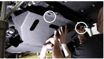
Secure the center and front plates to the support mount with the 2 remaining bolts, washers, and nuts.
