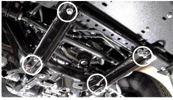
With a 12mm socket, remove the 4 bolts from each rear crash bar.
