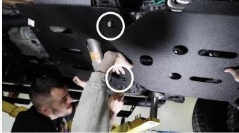
While supporting the plates, begin loosely securing the center plate to rear so that the center holds 'up' the rear, with 2 of the larger bolts, washers, and nuts with a 17mm socket and 6mm hex key.
