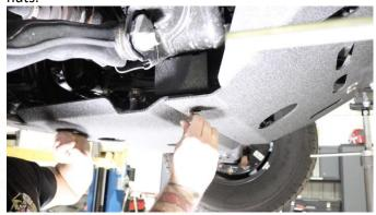
Each plate, from front to rear, should be supporting the next. Once the plates are in place, tighten down the button head bolts with a 17mm socket and 6mm hex key. Tighten the front factory bolts with an 18mm socket.
