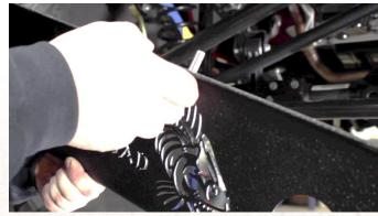
With your factory skid plate mounting bolts, secure the two plate brackets to the frame with a 16mm socket.
