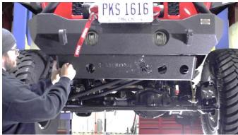
Install the included hardware into the remaining 5 skid plate and Mako bumper holes. With a 5mm allen key and a 13mm wrench, secure the skid plate
