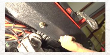
Install the support brackets into the factory tow hook locations. Notice how one of the holes in the frame protrudes. Use the included spacer on the hole that is not raised, and install the brackets using the factory hardware, and the included nuts into the bottom holes of the bumper brackets.
