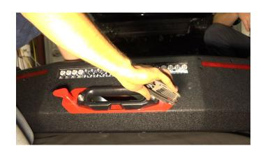
Insert the included stud plates into the bumper brackets, and use the plastic retainers to keep them from falling out. The large plate goes behind the top two holes, and the small single stud goes behind the outer corner hole.
