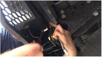
Adjust the height of the bumper as desired while making sure the tailgate doesn't hit, and tighten down the hardware.
