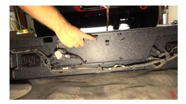
Install your factory license plate lights and trailer plug, and be sure to not over tighten the factory hardware.
