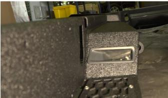
Look to see where your vehicle's exhaust pipes are located. Depending if you have a dual exhaust, remove the included exhaust covers accordingly.
