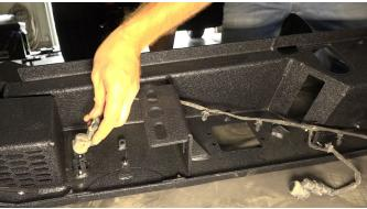
Install your pod lights with the included M6 hardware and a 4mm wrench and 10mm socket. Flush mounted lights (lights with a face plate) may be secured normally, but cube lights will require the included light brackets.
