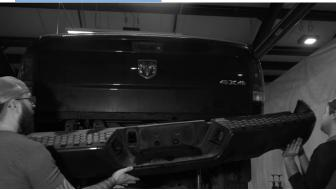
Remove the sensors and sensor wiring harness. Remove the trailer plug. Remove the license plate lights.
